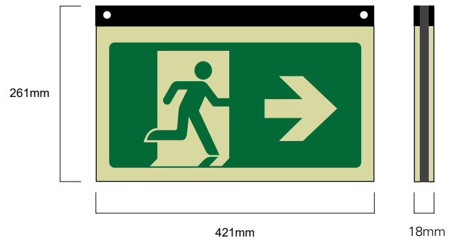
Diagram: Based on 24m EOS Exit Sign
